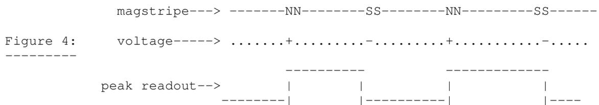
The "peak readout" square waveform is critical. Notice that the voltage peak remains the same until a new flux reversal is encountered.
