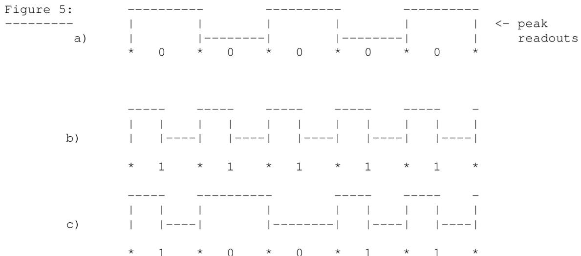
There you have it. Data is encoded in "bit cells," the frequency of which is the frequency of '0' signals. '1' signals are exactly TWICE the frequency of '0' signals. Therefore, while the actual
