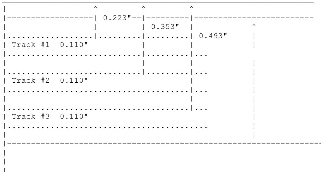
You can see the exact distances of each track from the edge of the card, as well as the uniform width and spacing. Place a magstripe card in front of you with the magstripe visible at the bottom of the card. Data is encoded from left to right (just like reading a book). See Figure 9.
